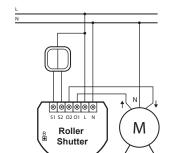
Fig.1 Wiring diagram for the Roller Shutter Controller
